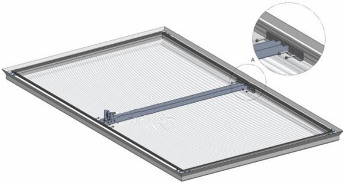
Fig. 15. Assembly of the leaf crossbar.
